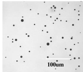
**Fig. 8** Jetted Droplets collected on the slide.
