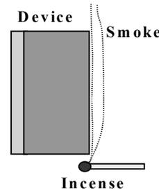
**Fig. 5** Set-up to test the air jet.
