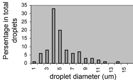
**Fig. 9** Droplet size distribution for the jetted water.
