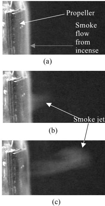
**Fig.12** Pictures showing the air jets produced by the propeller.
