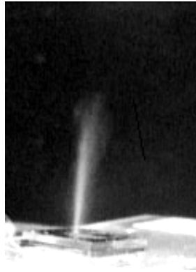
Fig. 7 Liquid jet stream produced by the liquid/air propeller.
