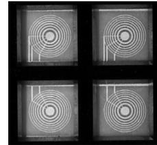
**Fig. 10** A 2 x 2 jet array for micropropulsion.
