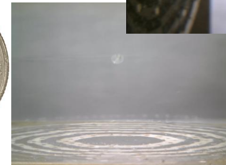
Trapping of Zebrafish Egg (1 mm in diameter, 1.4 mg in weight) with Acoustic Tweezers
